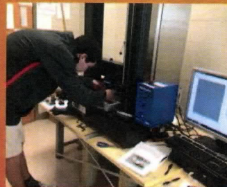
Measurement of deflections using ADMET MTEST Quattro Mechanical Testing System located at VSU Engineering Laboratory
