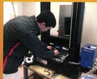
Measurement of deflections using ADMET MTEST Quattro Mechanical Testing System located at VSU Engineering Laboratory
