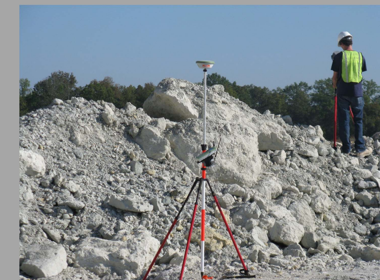
Scan Site 1: GPS set-up
