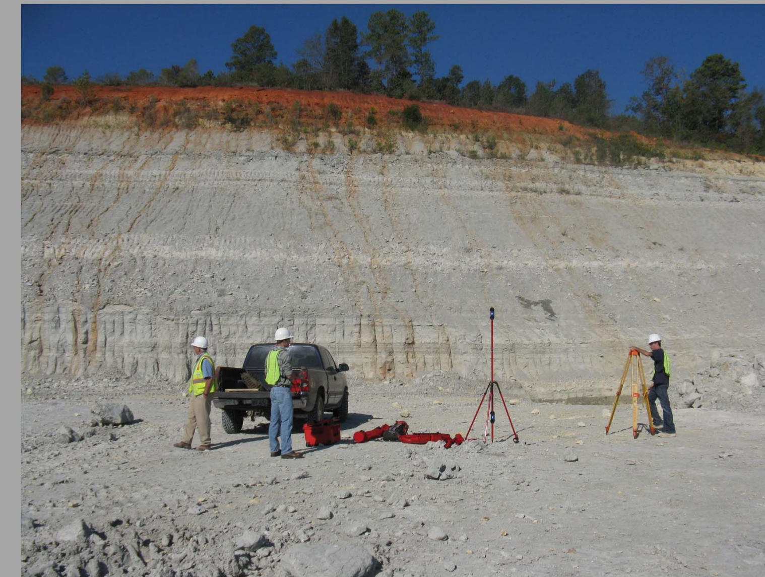
Scan Site 1: LiDAR scanner set-up
