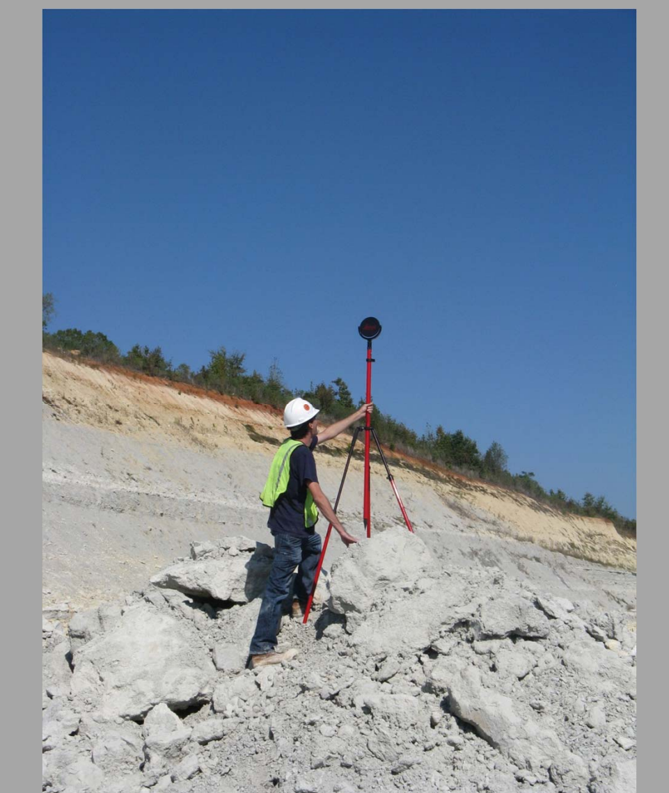
Reflector target set-up
