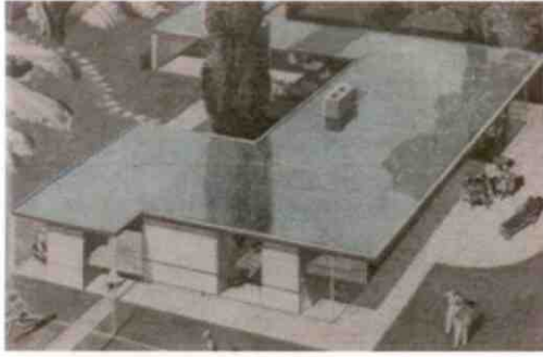
Inches-deep lake on roof already cools Southern homes and may become important air-conditioning method.
