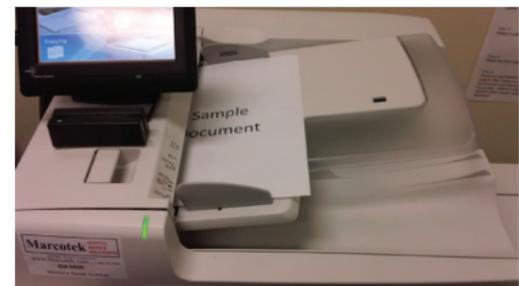
**Step 8** Press the **Start** button located on the bottom right of the touch screen to begin scanning to email.
